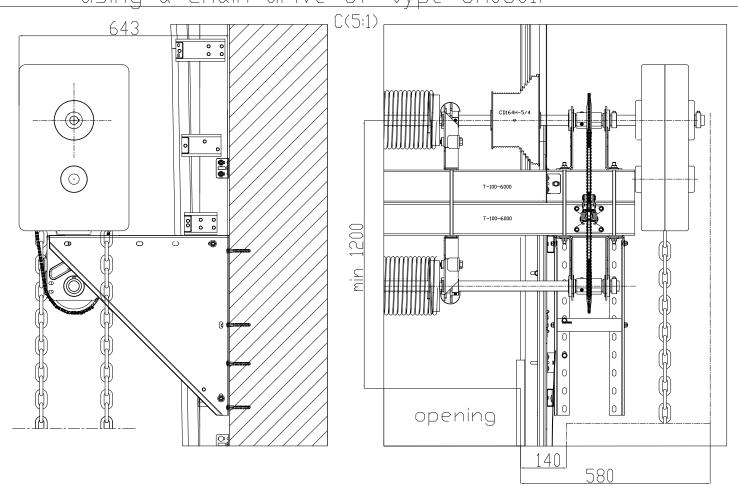
Additional parameters of the opening when using an electrical drive fixed on the door shaft
