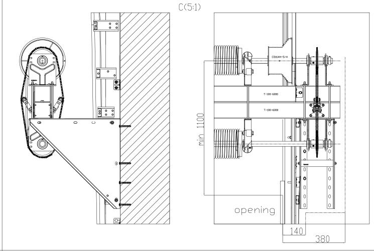
Additional parameters of the opening when using a chain drive of type CH0501.
